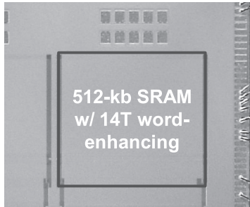
Fig. 13 Chip micrograph of the 512-kb SRAM macro with 14T word-enhancing scheme.
