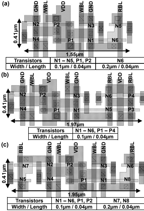
Fig. 4. Cell layouts of (a) 8T, (b) 10T-S, and (c) 10T-D SRAMs, in a 45-nm process technology.
