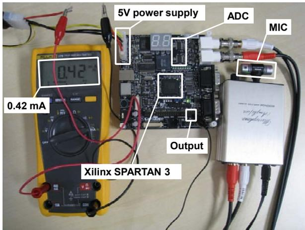
Fig. 5. FPGA board with a microphone and a current tester.
