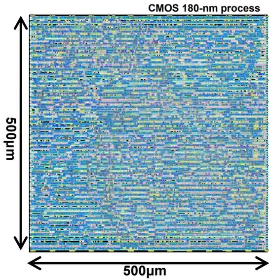
Fig. 6. Layout plot of the zero-crossing algorithm integrated using CMOS 0.18- $\mu\text{m}$  process technology.
