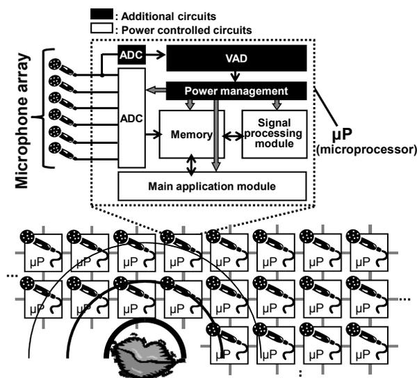
Fig. 1. Intelligent ubiquitous sensor network and a magnified block diagram showing a microprocessor and microphone array.
