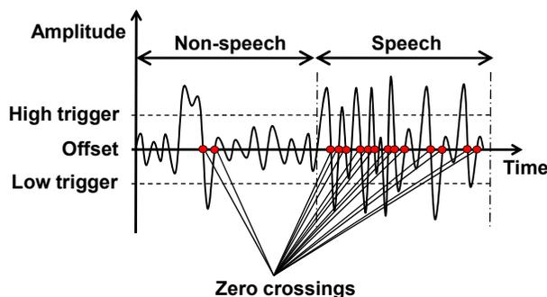
Fig. 2. Zero-crossing point example. The offset shows the direct current (DC) component.
