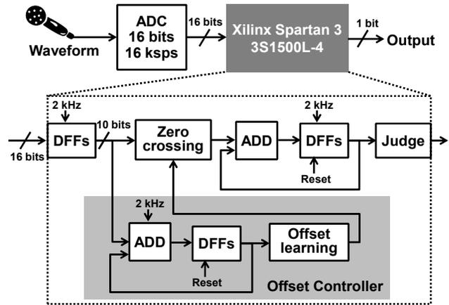
Fig. 4. Block diagrams of the integrated devices. The D flip-flop (DFF) circuits keep up each input data asynchronously.
