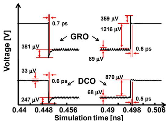
Figure 7 Noise waveforms on the power line of the oscillators.
