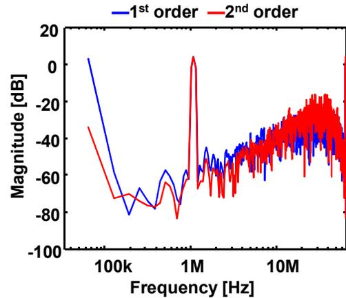
Figure 6 Output spectra of the first- and second-order noise shaping TDCs.
