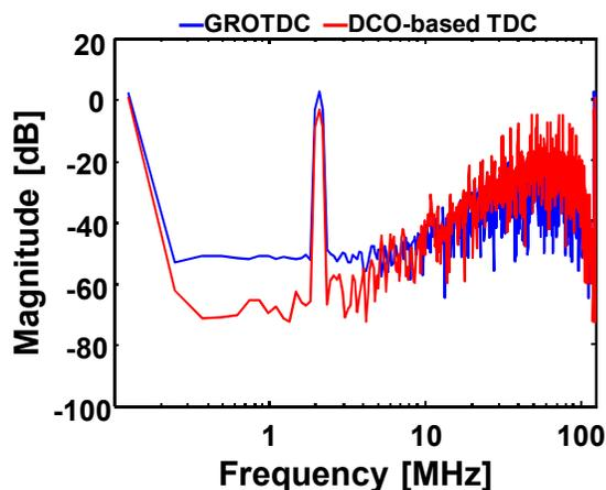
Figure 8 Output spectra of the conventional GRO-TDC and our proposed TDC both with second-order noise shaping.
