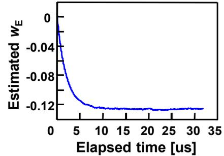
Figure 5 Learning curve of the LMS filter for coefficient estimation.
