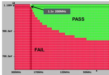
Fig. 10 Shmoo plot generated using a log tester.
