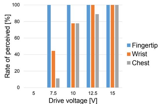
Fig. 10. Experimental result of required voltage to perceive haptic actuation.
