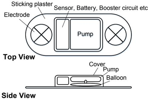
Fig. 5. Wearable device with PZT pump actuator.
