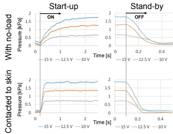
Fig. 7. Inner pressure transition of balloon at start-up and stand-by: (a) with no-load and (b) contacted to skin conditions.
