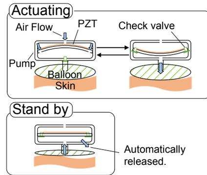
Fig. 3. Structure of proposed actuator using PZT pump.
