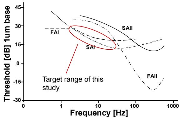
Fig. 2. Relation between stimulus frequency and sensitive threshold of displacement for each receptors. The original figure is presented in Ref. [5].
