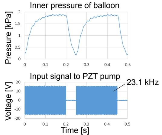
Fig. 8. Measured inner pressure of balloon while tactile stimulus generation. The balloon is contacted to skin.
