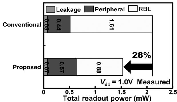
Fig. 19. Total readout power in 100-MHz operation.
