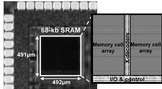
Fig. 16. Chip micrograph and its layout.
