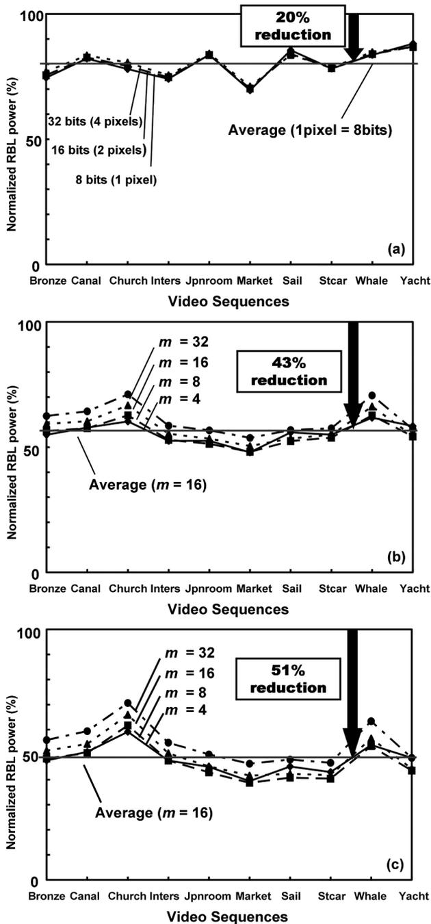
Fig. 8. Normalized RBL powers in (a) the original image only with majority logic, (b) the original image with both majority logic and data-bit reordering, and (c) the reconstructed image with both majority logic and data bit reordering. For this figure, 100% denotes a case of the conventional two-port SRAM.
