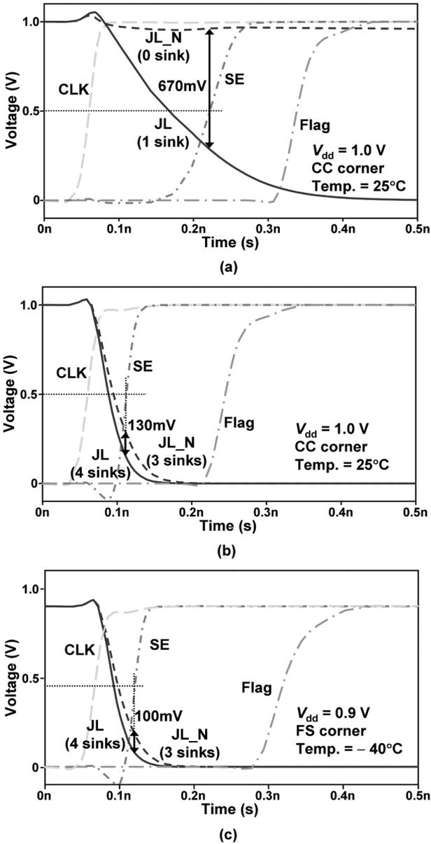
Fig. 14. Operation waveforms in a write circuit for which the numbers of “1”s and “0”s are seven and nine, respectively: (a) the case with one sink path on JL and zero sink path on JL\_N; (b) the case with four sink paths on JL and three sink paths on JL\_N; (c) the case with four sink paths on JL and three sink paths on JL\_N at the worst-case PVT variation.
