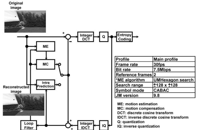
Fig. 7. H.264 encoding process and simulation conditions.
