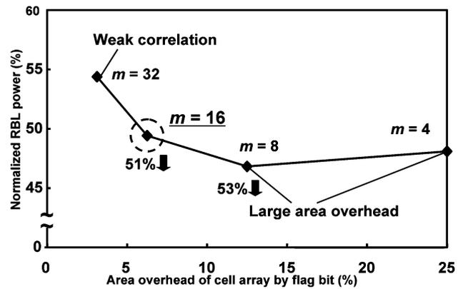
Fig. 9. Normalized RBL power versus area overhead of a memory cell in the proposed SRAM used as a reconstructed-image memory. The area overhead is  $1/m$  because the flag bit is appended to every  $m$  bits.
