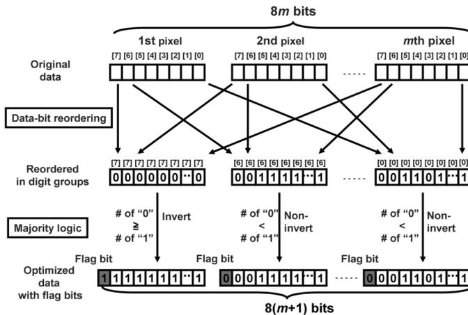
Fig. 6. Combination of data-bit reordering and majority logic.
