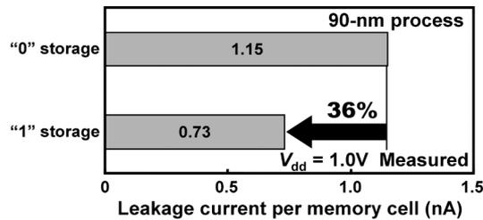
Fig. 17. Measured leakage current per memory cell.
