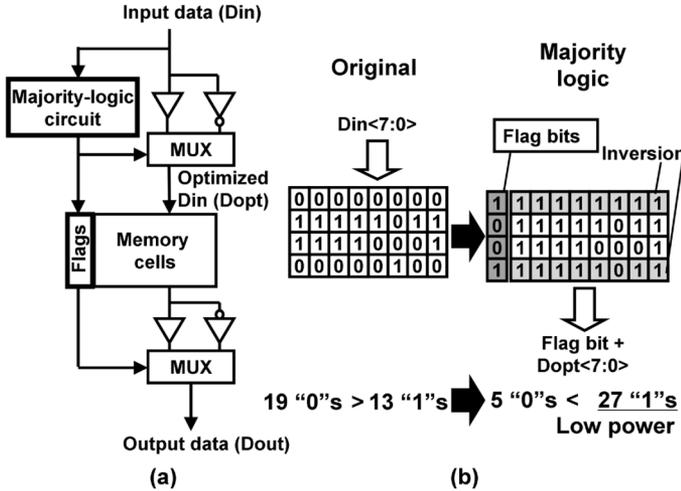
Fig. 2. Majority-logic circuit: (a) block diagram and (b) concept of flag bit.
