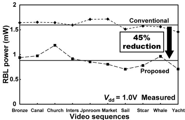
Fig. 18. Measured RBL power in 100-MHz operation.
