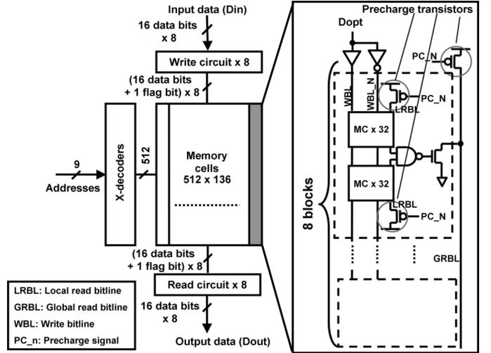
Fig. 12. Block diagram of the proposed 68-kbit SRAM.
