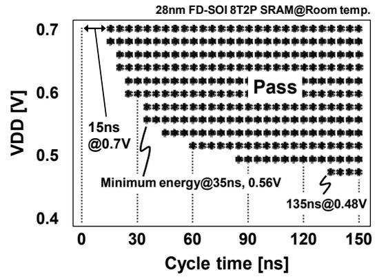
Fig. 7. Measured Shmoo plot in read operation.
