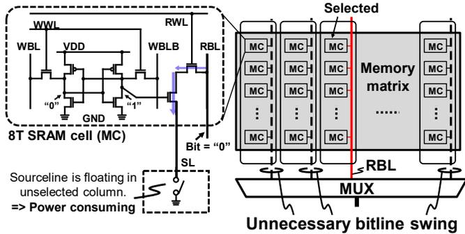
Fig. 1. Conventional 8T memory matrix with SSLC scheme. SLs are floating due to single nMOS switch; it consumes unnecessary energy.
