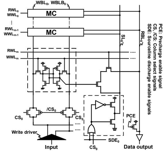
Fig. 8. Schematic of proposed 8T dual-port SRAM with SSD scheme.
