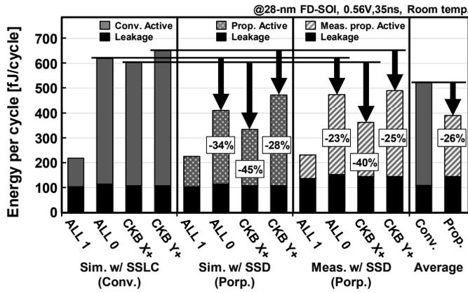
Fig. 9. Simulated and measured energy comparisons between conventional SSLC scheme and proposed SSD scheme in read operation.
