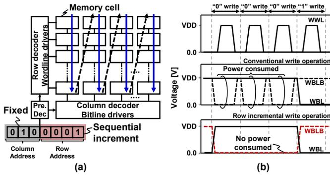
Fig. 5. Consecutive memory access in video processing: (a) Block diagram and (b) waveforms in write operation.
