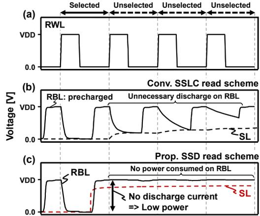
Fig. 3. Operating waveforms of proposed SSD scheme in read operation.
