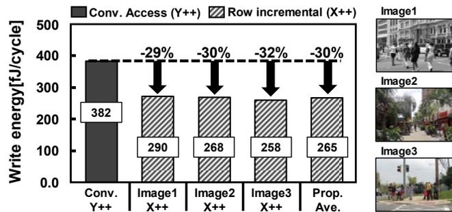
Fig. 10. Impact of incremental accesses in write operation.
