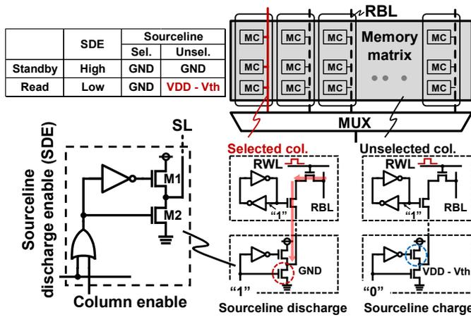
Fig. 2. Concept of proposed selective sourceline drive (SSD) scheme in read operation.
