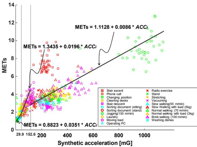
Fig. 2. Relation between measured synthetic acceleration and METs. METs is calculated from measured  $\dot{V}O_2$ .
