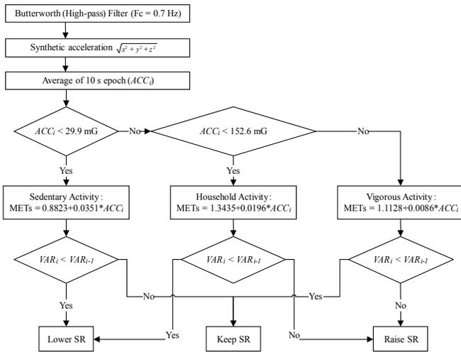
Fig. 1. Flow chart of proposed METs estimation algorithm.
