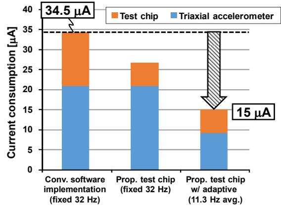
Fig. 9. System-level total current consumption.
