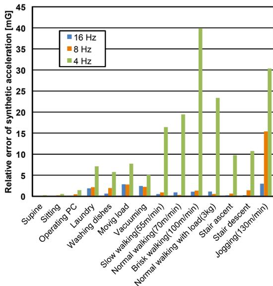
Fig. 3. Relative error of synthetic acceleration compared with 32-Hz fixed sampling rate in each activity.
