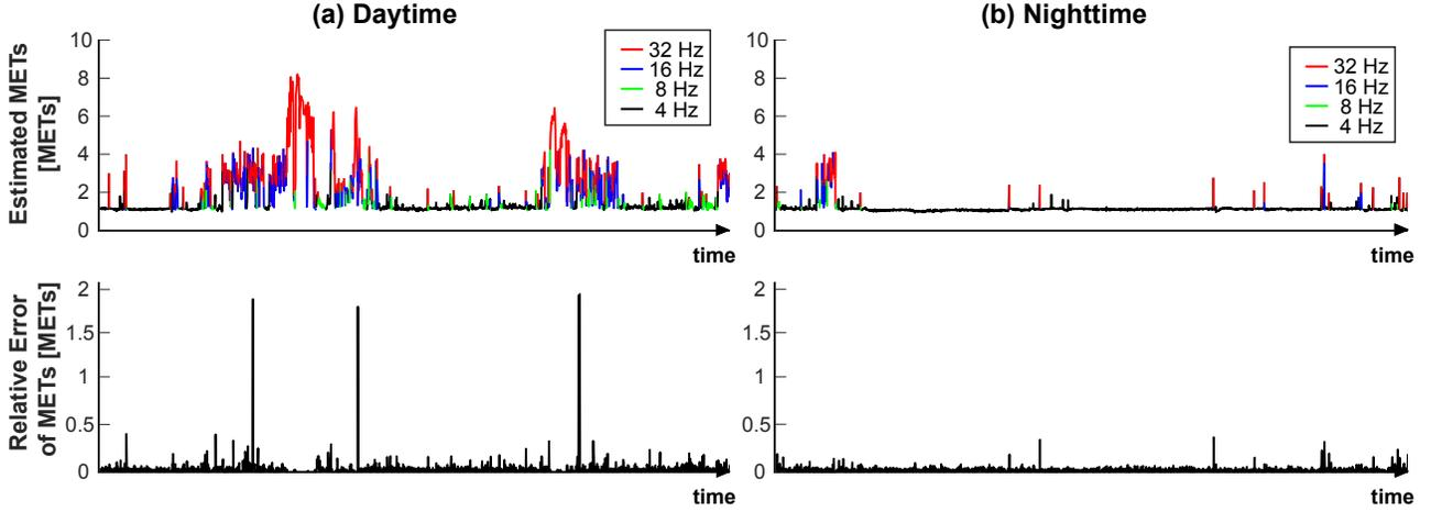
Fig. 5. Estimated METs and relative error from long-term measured acceleration using adaptive sampling: (a) in daytime and (b) at nighttime.
