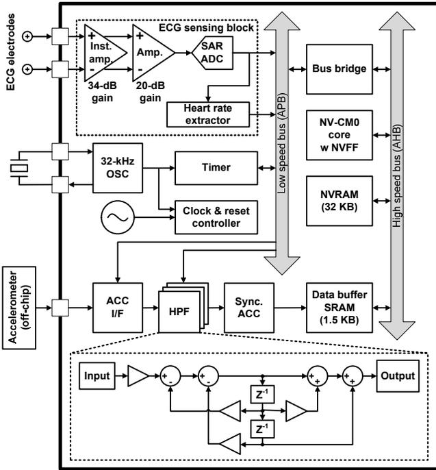
Fig. 6. Block diagram of the proposed METs estimation device.
