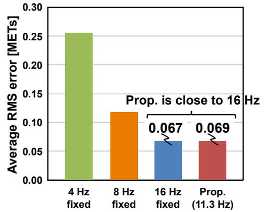
Fig. 4. Average root-mean-squared error of METs with proposed algorithm and at fixed rates, compared with METs values at 32-Hz fixed rate. METs are calculated from 24-hour acceleration data of six subjects.
