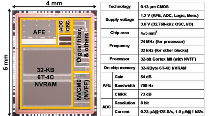
Fig. 7. Test chip micrograph and specifications.
