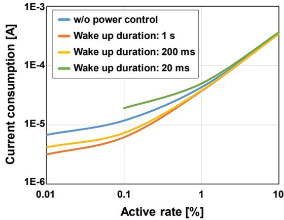
Fig. 8. Current consumption of non-volatile CPU.
