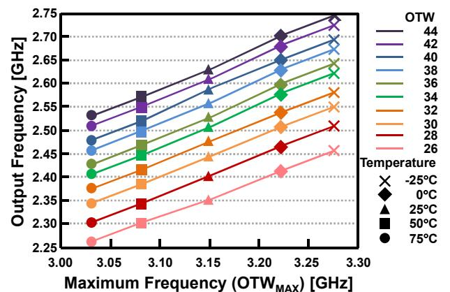
Figure 9. Temperature characteristics of DCO in measurements.
