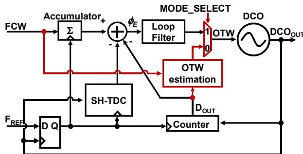
Figure 6. ADPLL with the proposed architecture.
