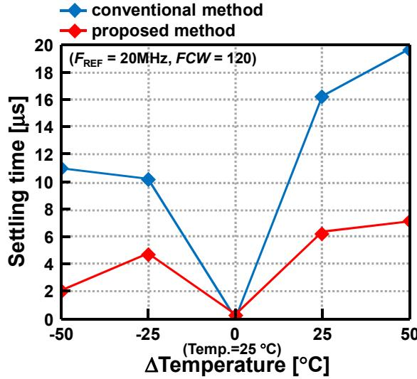
Figure 11. Simulation result of settling time.
