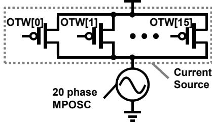
Figure 1. Schematic of digitally controlled oscillator (DCO).
