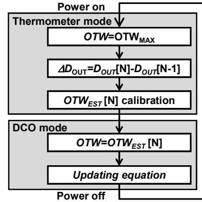
Figure 5. Calculation flow of temperature compensation.
