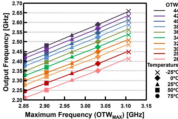
Figure 2. Simulated temperature characteristics of DCO.
