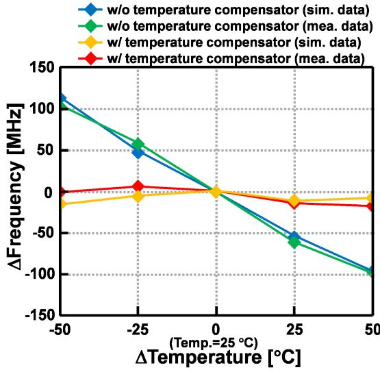
Figure 10. Simulation result of temperature compensation.
