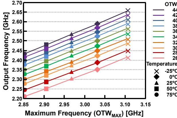
Figure 2. Simulated temperature characteristics of DCO.
