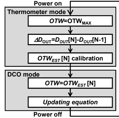
Figure 5. Calculation flow of temperature compensation.
