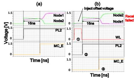
Fig. 10 (a) Recall operation waveforms of faulty cell (a) without and (b) with the proposed test scheme.
