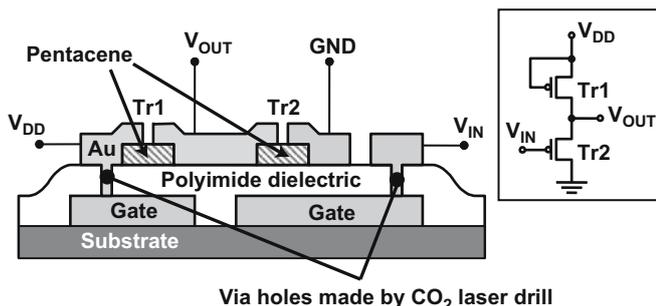
**Fig. 1** Cross-sectional illustration of flexible organic transistors on a polyimide base film, and schematic diagram of inverter circuit (*inset*). The thickness of each layer is: polyimide base film 75  $\mu\text{m}$ , gate electrode 100 nm, polyimide gate-insulating layer 900 nm, pentacene 50 nm, and source-drain electrode 40 nm
