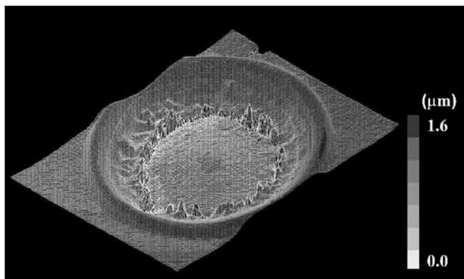
**Fig. 2** 3D contour of a via hole formed by a laser drilling machine (viewed with a laser microscope)
