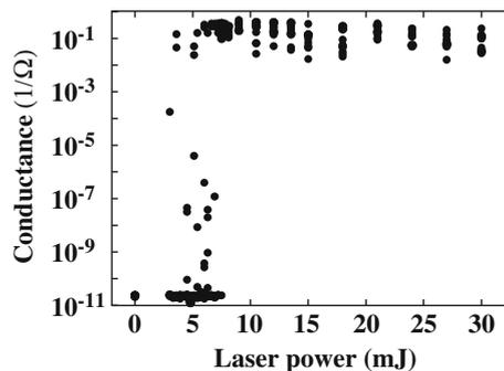
**Fig. 3** Dependence of conductance through via holes on input laser power
