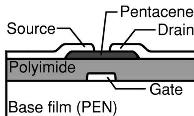
FIG. 1. (a) The cross-sectional illustration of transistors on a PEN-based film. The thickness of each layer is as follows; a PEN-based film 125  $\mu\text{m}$ , gate electrode 150 nm, polyimide gate dielectric layer 990 or 540 nm, pentacene channel layer 50 nm, and source–drain electrode 60 nm.
