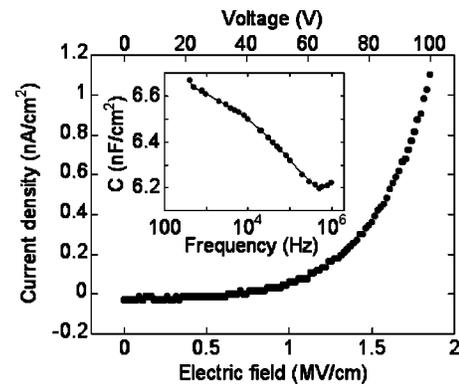
FIG. 3. Current leakage for 540 nm polyimide insulators is measured as a function of electric field. Capacitance is shown at various frequencies on the same structures as the inset.
