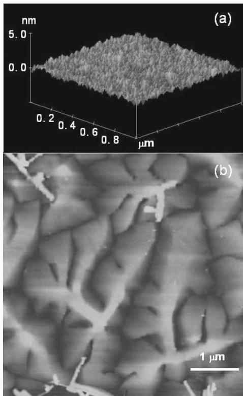
FIG. 2. (a) The surface of polyimide gate dielectric layers prepared on a PEN-based film is characterized by AFM. (b) The surface of pentacene thin films deposited on polyimide gate dielectric layers is also characterized by AFM.
