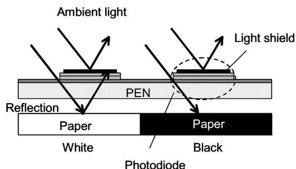
Fig. 5: A principle of imaging with the present sheet image scanner, which is placed onto paper with white and black regions.
