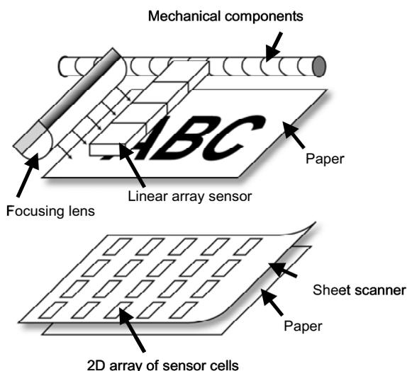
Fig. 4: Schematic illustrations of a conventional scanner and the present sheet image scanner. A conventional scanner consists of a linear array of sensors and that of light sources. The new scanner consists of a two-dimensional array of organic photodiodes coupled with organic transistors, which can be read out electrically by the organic transistors.
