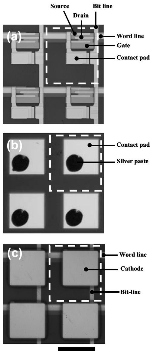
Fig. 3: (a) A magnified image of four transistors before integrating with organic diodes. The channel length  $L$  and width  $W$  are  $18 \mu\text{m}$  and  $400 \mu\text{m}$ , respectively. (b) A magnified image of four contact pads with silver paste islands before laminating organic transistor films and organic diode films. (c) A magnified image of four sensor cells integrating organic transistors and organic photodiodes. Scale bar is  $500 \mu\text{m}$ .
