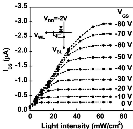
Fig. 6:  $I_{DS}$  vs. light intensity is measured for one sensor cell of the 36-dpi integrated devices with a different  $V_{GS}$  bias. The power supply  $V_{DD}$  is  $-2 \text{ V}$ .
