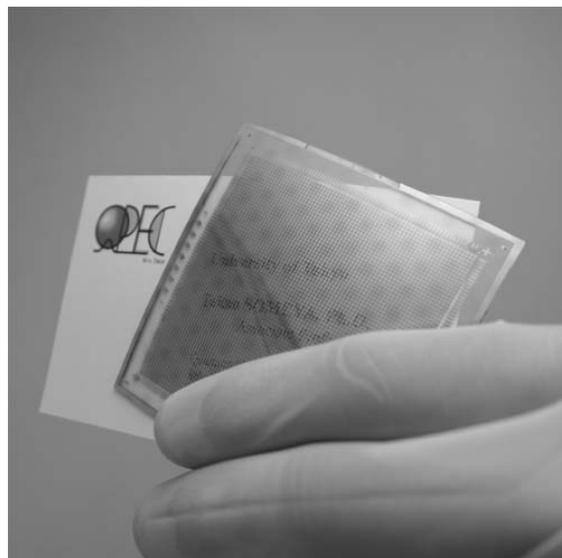
Fig. 1: An image of the manufactured large-area, flexible, and lightweight *sheet image scanner* consisting of organic transistors and organic photodiodes, which is placed on a business card under ambient light for capturing image.
