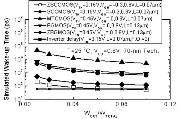
Fig. 8. Simulated wakeup times of ZSCCMOS, SCCMOS, BGMOS, MTCMOS, and ZBGMOS with 70-nm BPTM. The simulation is done with  $T = 25^{\circ}C$  and  $V_{DD} = 0.6V$ .
