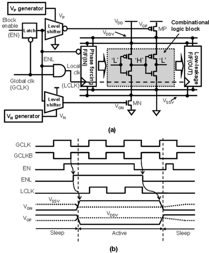
Fig. 4. (a) ZSCCMOS block activation scheme with the combinational logic block, F/Fs, and the control logic of the clock gating. (b) Waveforms of Fig. 4(a).
