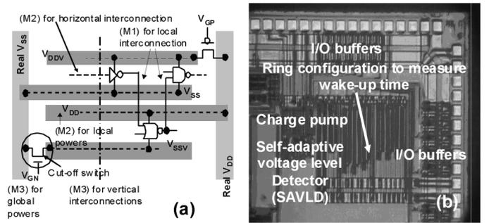
Fig. 11. (a) Layout of ZSCCMOS with power switches and virtual and real power lines. (b) Test chip micrograph with 0.6- $\mu m$  technology.
