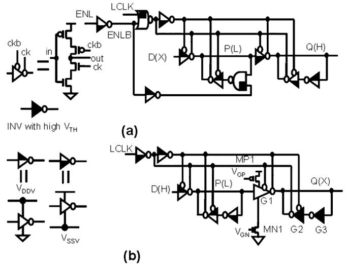
Fig. 5. (a) Schematic of input flip-flop with phase-forcing circuit. (b) Schematic of low-leakage output flip-flop.
