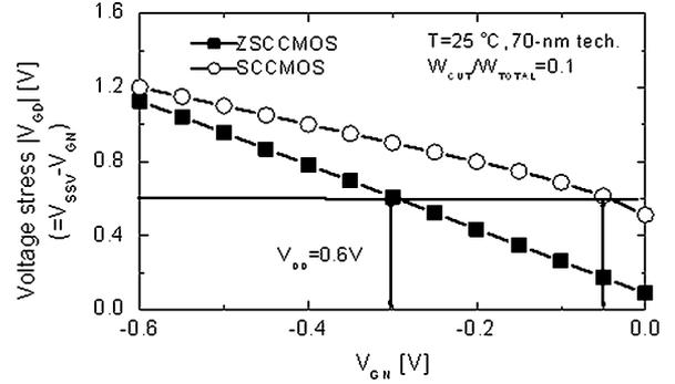
Fig. 3. Voltage stress plot of the power switches of SCCMOS and ZSCCMOS. Here,  $V_{GD}$  is the gate-drain voltage of MN1 in Figs. 1 and 2.
