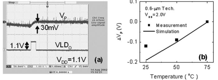
Fig. 12. (a) Measured operating waveforms of  $V_P$  (positive voltage) generator. (b) Measured  $V_P$  with varying temperature.
