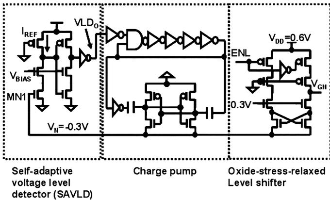
Fig. 7.  $V_N$  (negative voltage) generator for NMOS power switch.
