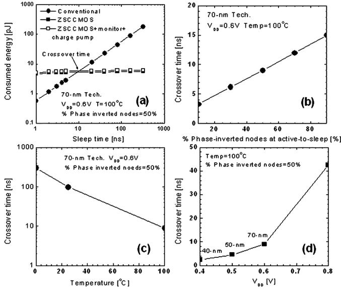
Fig. 10. (a) Energy consumption with increasing sleep time. (b) Crossover time with varying percentage of phase-inverted nodes at the active-to-sleep transition. (c) Crossover time with varying temperature. (d) Crossover time with various process nodes.
