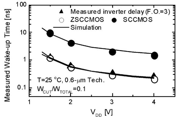
Fig. 9. Measured wakeup times of SCCMOS and ZSCCMOS in 0.6- $\mu m$  technology.
