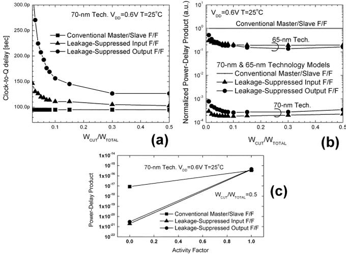
Fig. 6. (a) Clock-to-Q delay simulation of various F/Fs. (b) Power-delay product simulation of various F/Fs. (c) Power-delay product simulation with varying activity ratios. Here, the  $V_{TH}$ s of 70-nm and 65-nm BPTMs are 0.06 and 0.05 V, respectively, and the temperature is  $25^{\circ}C$ .
