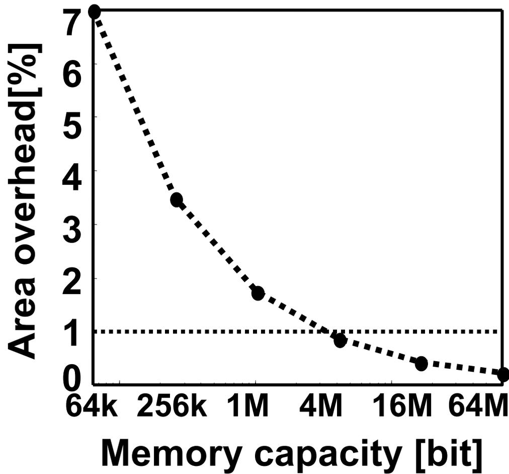
**For 4M bit SRAM, area overhead is less than 1%.**
