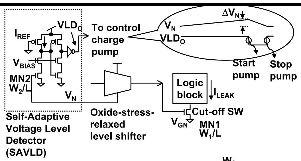
• Self-adaptively adjusting  $V_N$  as  $I_{LEAK} \frac{V_2}{W_A} = I_{REF}$
