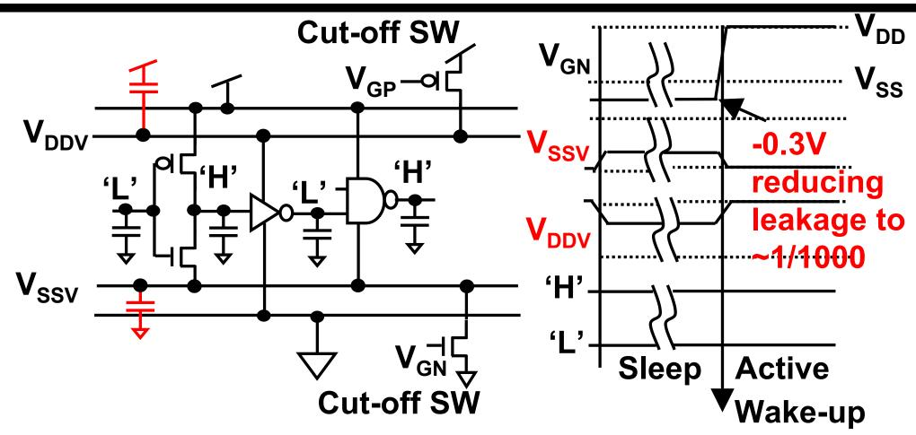
Small voltage change of V<sub>SSV</sub> and V<sub>DDV</sub> due to reversesource biasing effect
