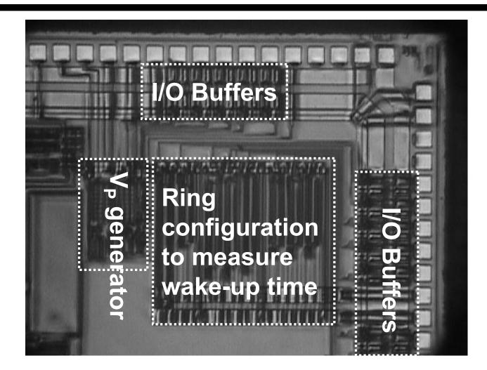
Fabricated in 0.6-µm CMOS technology
