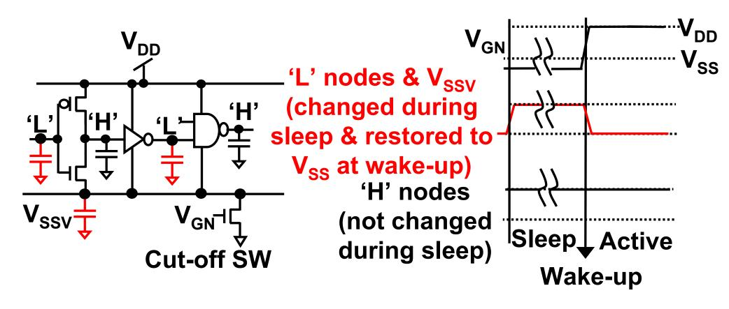
Full swing of 'L' nodes and V<sub>SSV</sub> nodes at wake-up
