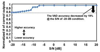
Fig. 7. The number of *correct* VAD outputs using the number of outputs from VAD as normalized criteria.
