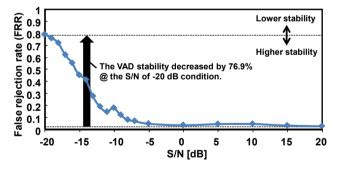
Fig. 9. The false rejection rate (FRR) in VAD outputs using the speech frames of the recorded condition as normalized criteria.
