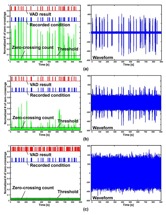
Fig. 10. Waveforms and zero-crossing results at (a) S/N=20 dB, (b) S/N=0 dB, and (c) S/N=-20 dB.
