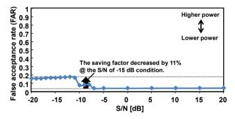
Fig. 8. The false acceptance rate (FAR) in VAD outputs using the number of non-speech frames of the recorded condition as normalized criteria.
