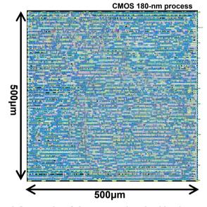
Fig. 6. Layout plot of the zero-crossing algorithm integrated using CMOS 0.18-µm process technology.
